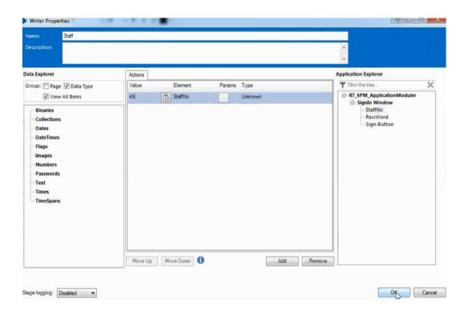
**Step 9:** Using another write stage to configure the Password.
