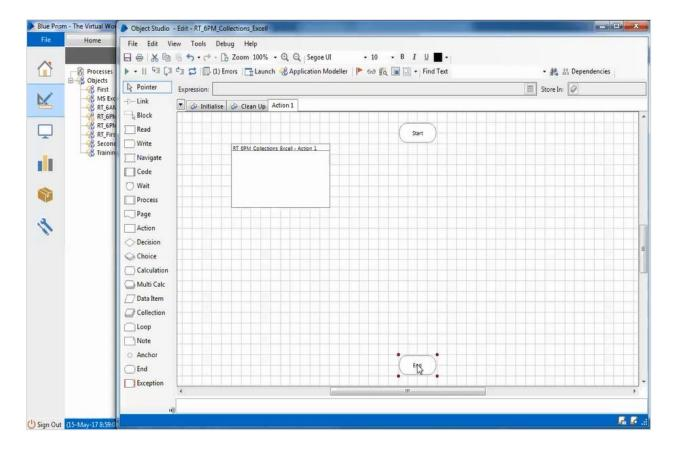
In the action tab, the start and end stages will be created by default with a link to them, select the link and delete, so that the actual stages can be implemented in it.
