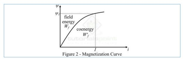
For a **linear electromagnetic system**, the energy stored in the magnetic field is given by,
