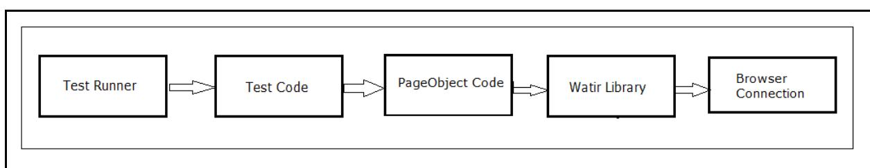
RSpec or Cucumber are involved in test runner and test code. The details about the website or UI testing can be broken down into page object which will have reference to Watir, wherein it will get the page locators to be used for testing. Watir, along with its webdriver, helps in connecting to the browser and carry out the test automation.
